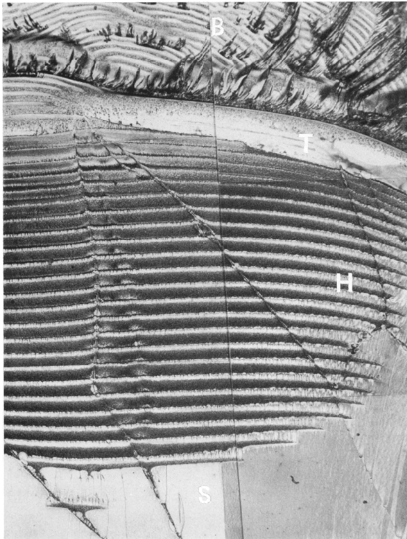
Figure 4 Surface of fracture of polystyrene formed at 90°C. Area S: slow crack propagation near median plane of craze; area T: transition belt where craze wedge breaks off along craze-bulk boundary; area B: field of banding, fast propagation; area H: alternating bands formed by viscous flow (light) and viscous rupture (dark). Composite photomicrograph; reflected light, \lambda = 546 \text{ nm} , \times 80 .
